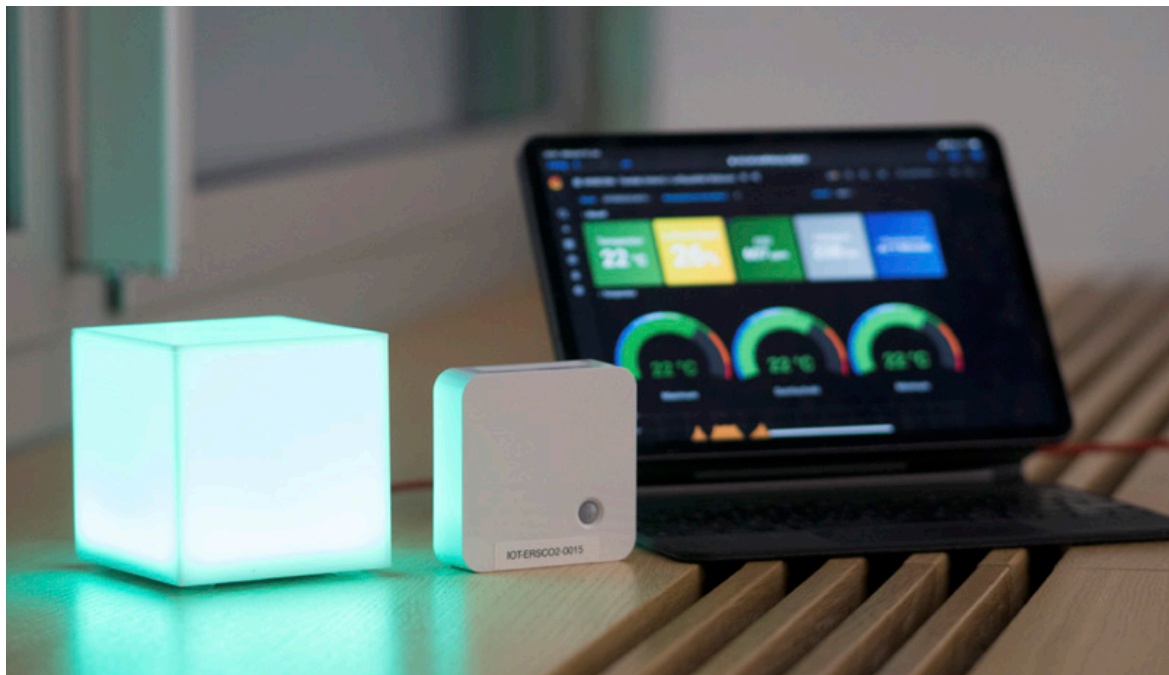
Figure 1 - LWOB.smart sensors, dashboard and LED cube - complete equipment for fully automated air measurement
